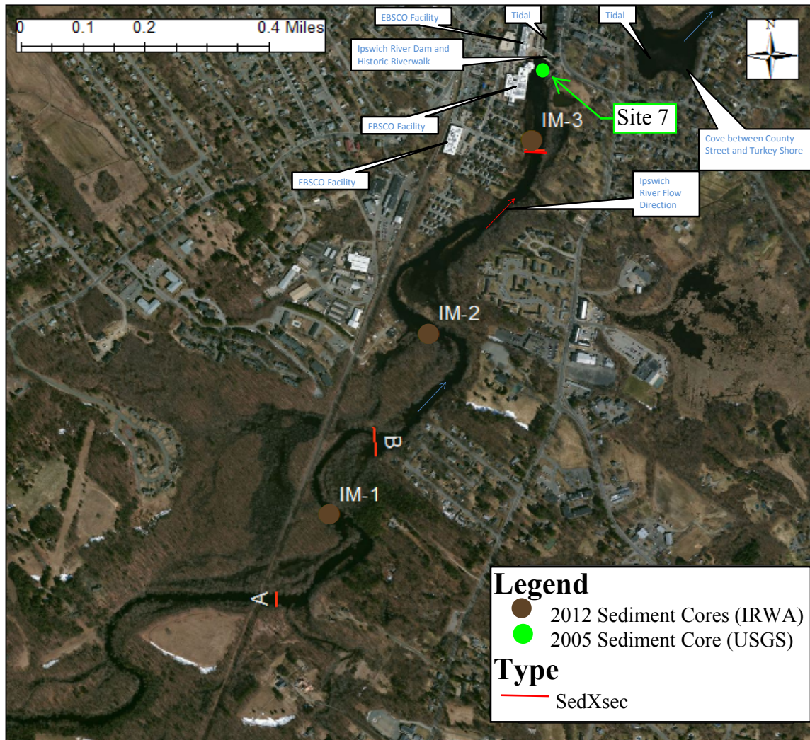
Figure: Sediment core locations and sediment depth cross sections from 2012 surveys of Ipswich Mills impoundme
