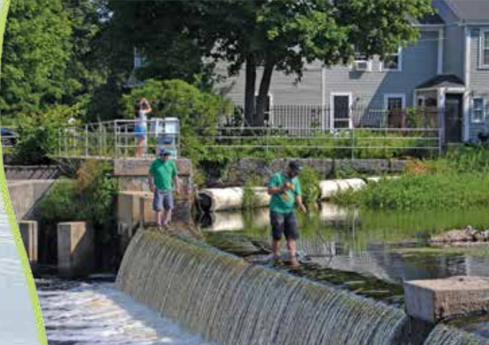
The survey crew from Norde-East Survey wades across the Ipswich Mills Dam spillway to make final depth and sediment measurements at the crest of the dam. They also recorded depth soundings in the human-made pond upstream of the Ipswich Mills Dam in Ipswich.
