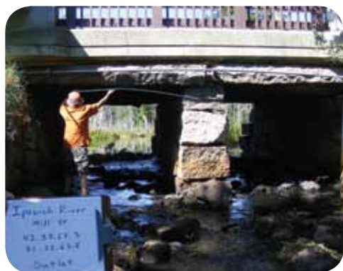
Will Finch measures the bridge at Mill St in Reading to see if it provides safe passage for fish and other wildlife or poses a threat for flooding. Photo: C. Sandberg
