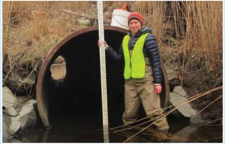
Kristen Thiebault completes one of the more than 100 assessments done using the new Tidal Stream Crossing protocol. The protocol was developed in 2019 in collaboration with Scott Jackson and the North Atlantic Aquatic Connectivity Collaborative thanks to the Massachusetts Environmental Trust Grant program. Along with other data, the new protocol is a better model for assessing accessibility for fish passage in tidally influenced sites. Learn more ipswichriver.org/tidal-crossing-protocol .
