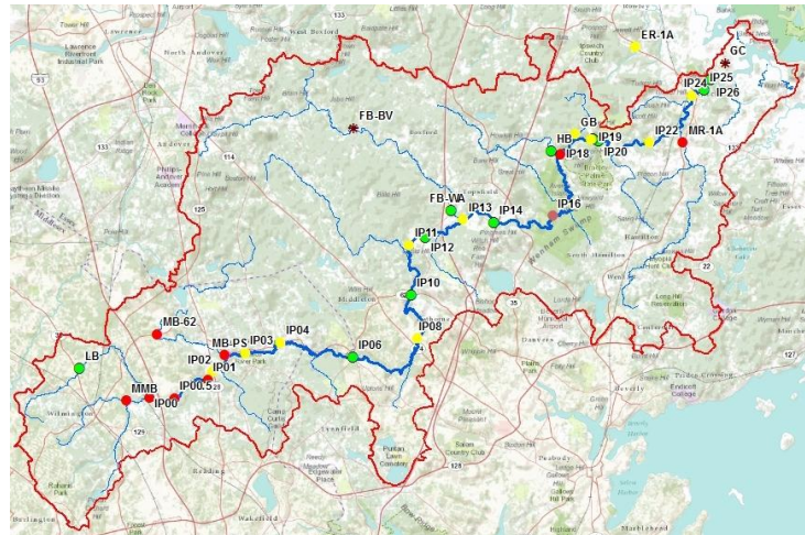
Figure 1. Average summer dissolved oxygen levels for 2011. Sites in red (< 3mg/L) represent a highly stressed environment for fish and other aquatic organisms.
