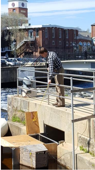
Figure 5. View of the counting board from the perspective of a fish counter standing on the walkway. The camera housing is on the left.
